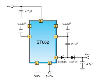
Evaluation circuit when  $V_{OUT}$  is greater than 12V
